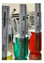
Year 8s made barometers and are using these to measure changes in pressure. By also recording the weather, they can determine a link between it and barometric pressure.
